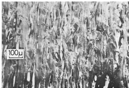
Fig. 8. Voided structure of 50 PE:50 PP drawn at 125°C.
